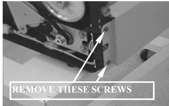
**Front Cover**-Remove the front panel by first removing the two end covers (see above) and then removing four (4) pan head screws (2 each side) securing the front panel to the chassis. Refer to the photo above right.
