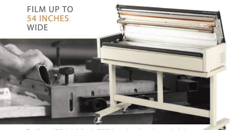
The Liberator XE Series is built using EXILE's innovative and proprietary technologies, including: Closed Loop Registration (CLR) control for accurate registration overlay, Multi-Level Pulsing (MLP) for superior dot quality, and Enhanced Nib Management (ENM) to provide smooth, high-quality images every time.
