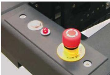
To shut down the machine, click **File > Exit** or just close the program window. After the program exits, press the emergency button at the right-hand side of the machine, and the computer can also be shut down if necessary.
