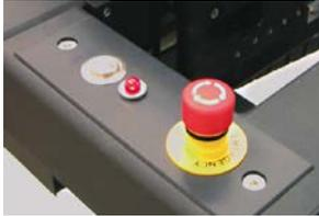
An emergency stop “panic button” is located in the right-hand side of the machine. It is a large, red button that can be pushed to remove all power from the machine. This is the safest way to insure that dangerous voltages are not present in the machine, but when this device is deactivated, the ink will solidify, and an unusually long time will be required to return the machine to service. To recover from an emergency stop, turn the button clock-wise and press the “Start” button below it.
