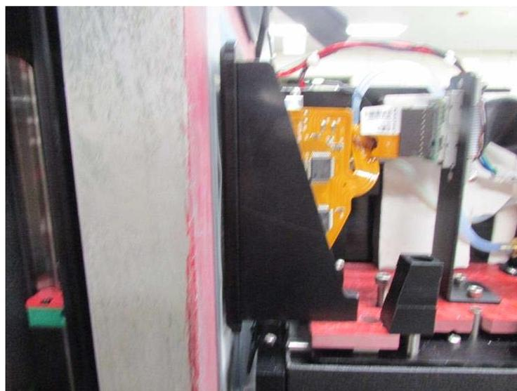
The two screws to the left of the printhead can be used for adjustment:
