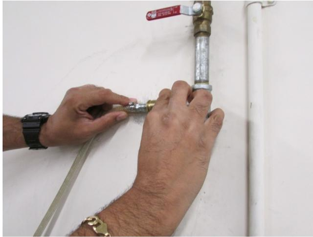
2. Insert the other end of the air hose into the valve next to the pressure gauge at the back of the printer.
