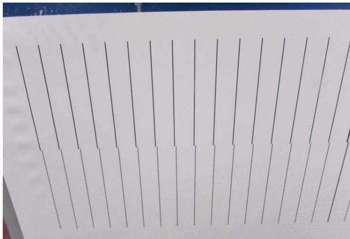
Note the vertical lines in the 2<sup>nd</sup> head section is disconnected (off to right) from the 1<sup>st</sup> section, instead of a seamless transition, and it's due to the tilting of the printhead.
