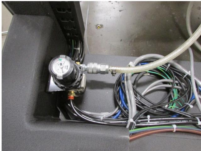
3. To feed air to the printer, open the valve on the wall pipe. Then pull upwards on the knob of the pressure gauge, and turn it clockwise until it reaches 45 psi. When set, press the knob down to lock it.
