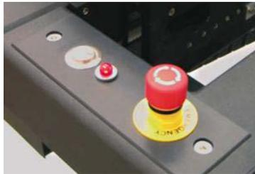
Rotating the emergency button clockwise and then pressing the “Start” button just below it will power up the machine. Then click on the “Spyder Control Panel” shortcut icon on the desktop to start the software. After the app is started, click the **Continue** button. The head assembly and drum support will move to the home position.
