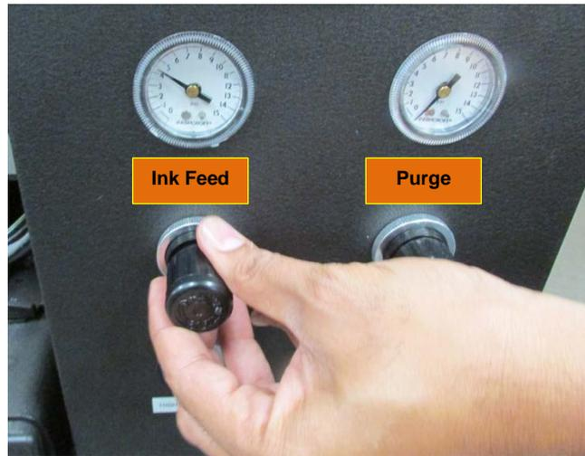
Verify that purge pressure gauge be ~4 psi. If not, it can be regulated by lifting the knob below the gauge and turning it right to increase or left to decrease the pressure. When finished, push the knob back down.
