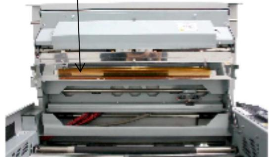
3. *The dirt cannot be seen visually on the head, but you can see any streak image on the film.*
